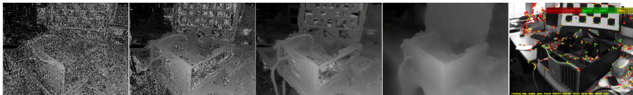
Figure 3. Incremental cost volume construction; we show the current inverse depth map extracted as the current minimum cost for each pixel row d_u^{min} = \arg \min_d C(u, d) as 2, 10 and 30 overlapping images are used in the data term (left). Also shown is the regularised solution that we solve to provide each keyframe inverse depth map (4th from left). In comparison to the nearly 300 \times 10^3 points estimated in our keyframe, we show the \approx 1000 point features used in the same frame for localisation in PTAM ([6]). Estimating camera pose from such a fully dense model enables tracking robustness during rapid camera motion.
