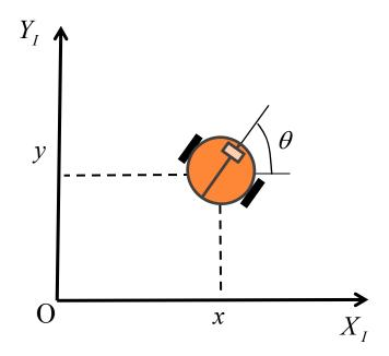
$$\begin{bmatrix} x_{1,t} \\ x_{2,t} \\ x_{3,t} \end{bmatrix} = g(x_{t-1}, u_t) = \begin{bmatrix} x_{1,t-1} + u_{1,t} \cos x_{3,t-1} dt \\ x_{2,t-1} + u_{1,t} \sin x_{3,t-1} dt \\ x_{3,t-1} + u_{2,t} dt \end{bmatrix}$$
