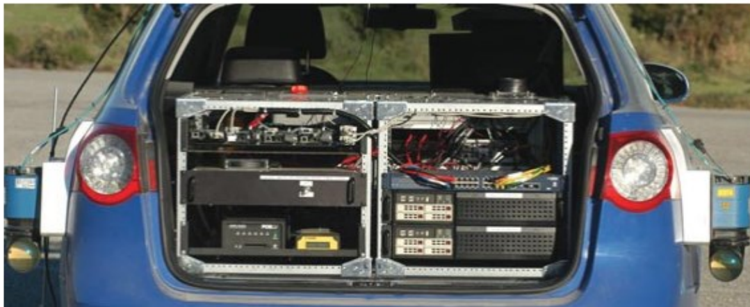
Figure 2. All computing and power equipment is placed in the trunk of the vehicle. Two Intel quad core computers (bottom right) run the bulk of all vehicle software. Other modules in the trunk rack include a power server for selectively powering individual vehicle components and various modules concerned with drive-by-wire and GPS navigation. A six-degree-of-freedom inertial measurement unit is also mounted in the trunk of the vehicle, near the rear axle.
